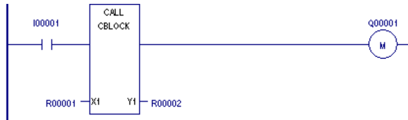
Figure 2: Invoking a C block from Ladder Program
